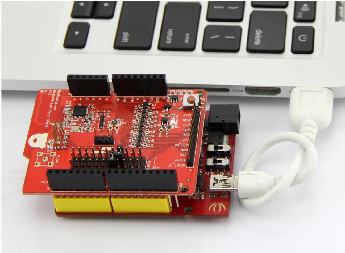
5. Check the Power LED on both Seedeino and BLE Shield 2 are lit up.
