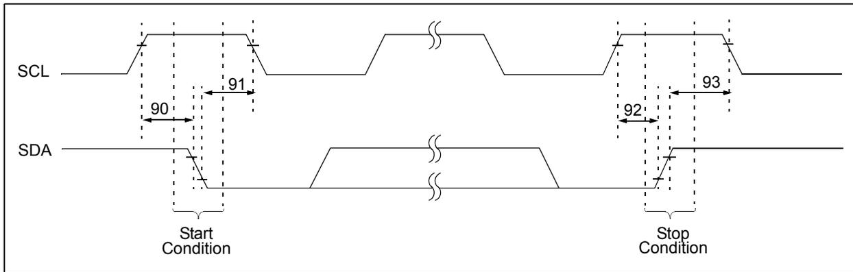
**FIGURE 2-4: I<sup>2</sup>C™ BUS DATA TIMING**
