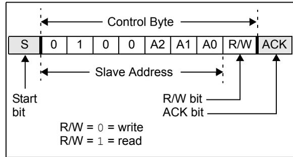
FIGURE 1-3: SPI CONTROL BYTE FORMAT
