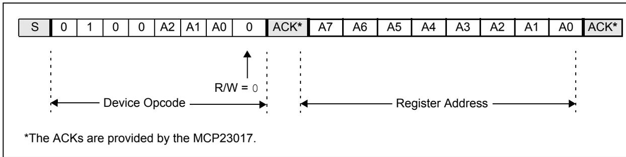
FIGURE 1-5: SPI ADDRESSING REGISTERS
