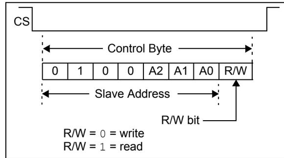
FIGURE 1-4: I<sup>2</sup>C™ ADDRESSING REGISTERS
